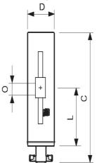
DimC max 52 mm DimD 0 mm DimD\_max 13 mm DimL\_min 22 mm DimL 23 mm DimL max 23 mm DimO 3 mm
